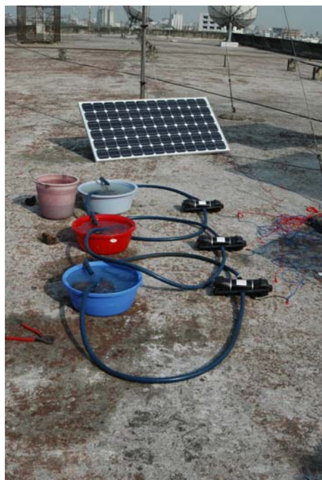
Fig 4. Multiple switched motor.
