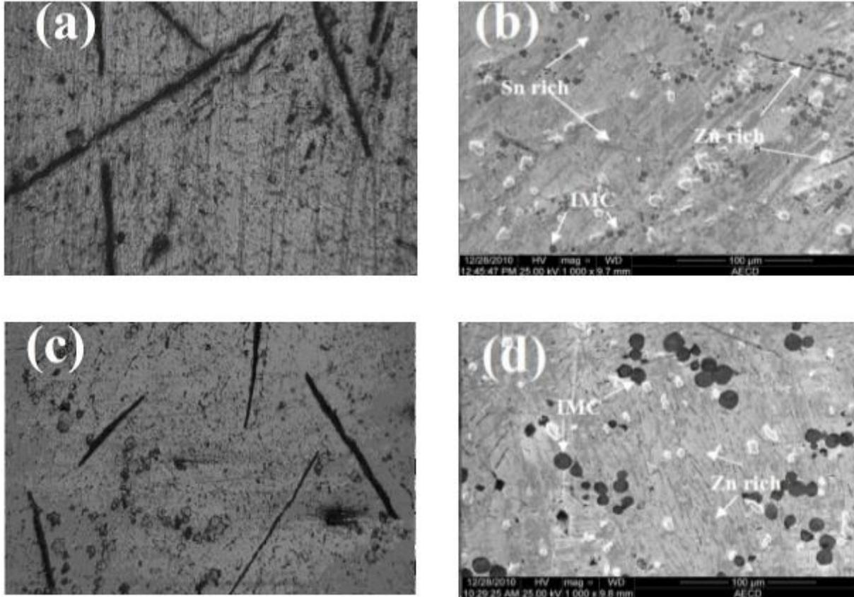
Fig. 3. (a) Optical micrograph of Sn-9Zn-2.0Al (b) SEM micrograph of Sn-9Zn-2.0Al (c) Optical micrograph of Sn-9Zn-4.0Al (d) SEM micrograph of Sn-9Zn-4.0Al
