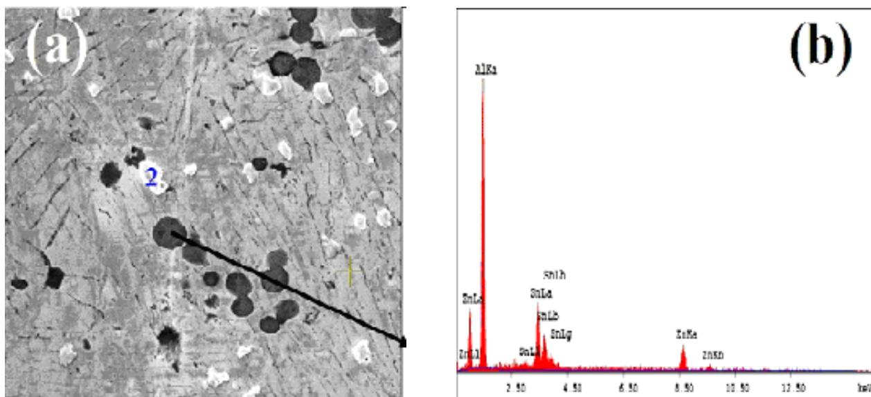
Fig 4. (a) The dark gray phases for Sn-9Zn-2.0Al alloy and (b) their quantitative analyses with EDX
