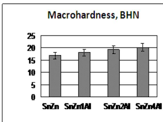
Fig 5. Brinell Hardness Number (BHN) for Sn-9Zn, Sn-9Zn-1.0Al, Sn-9Zn-2.0Al, and Sn-9Zn-4.0Al alloys.
