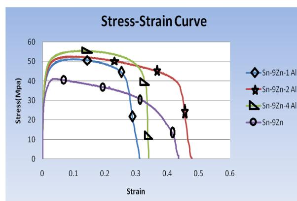
Fig 6. Tensile Stress-Strain curves of Sn-9Zn, Sn-9Zn-1.0Al, Sn-9Zn-2.0Al, and Sn-9Zn-4.0Al alloys.
