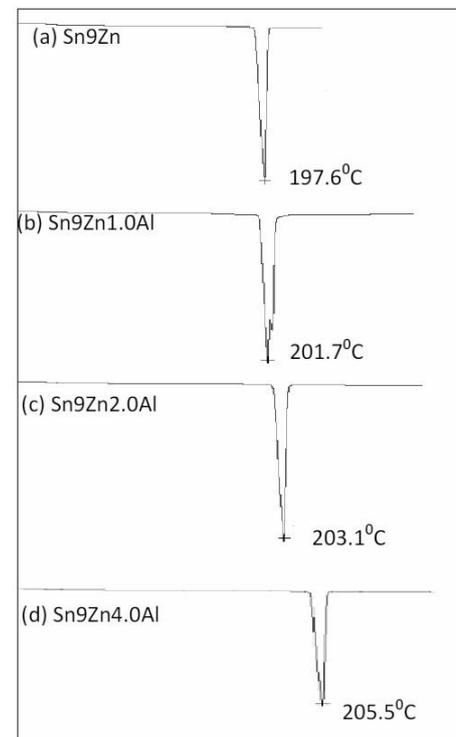
Fig 1. DSC curves of Sn-9Zn, Sn-9Zn-1.0Al, Sn-9Zn-2.0Al, and Sn-9Zn-4.0Al alloys
