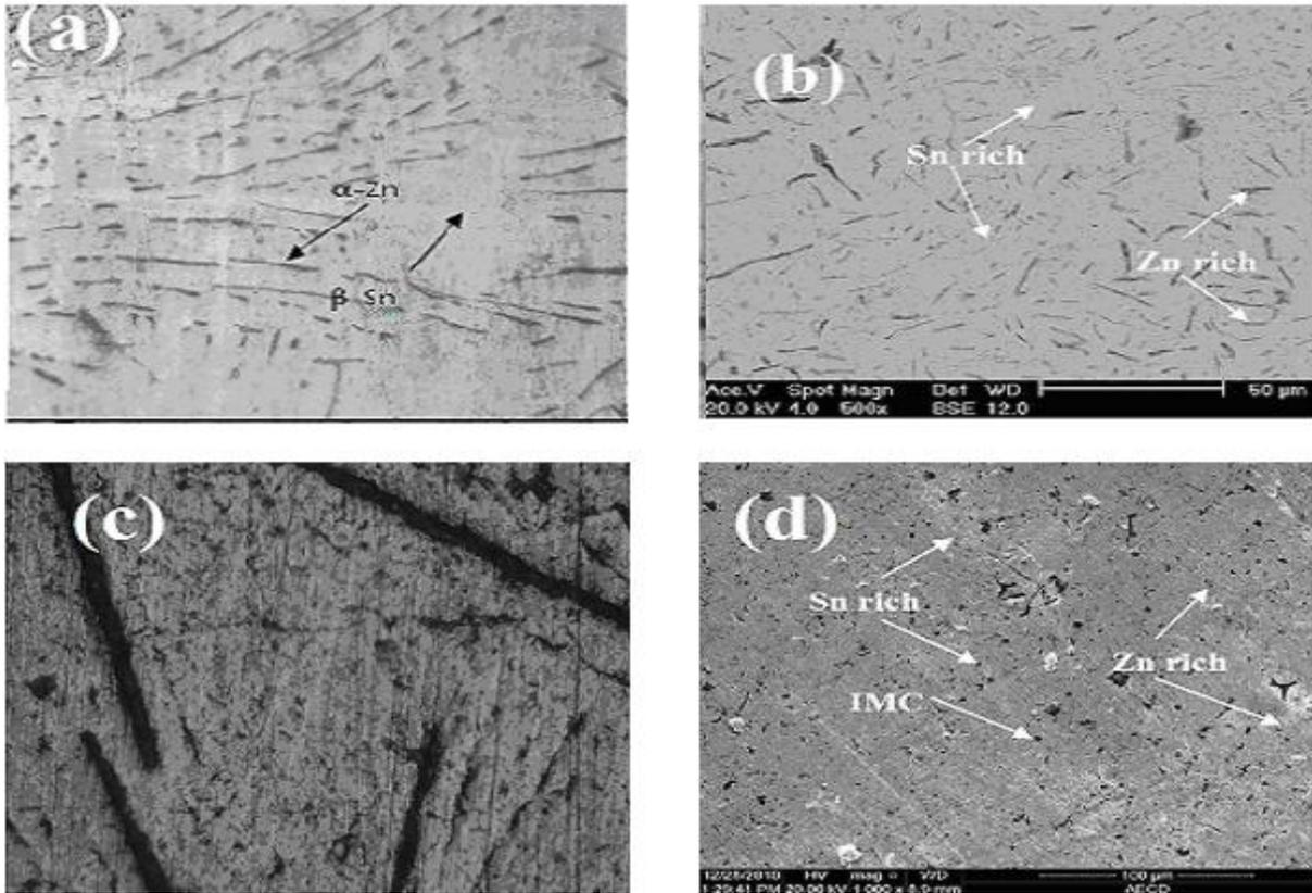
Fig 2. (a) Optical micrograph of Sn-9Zn (b) SEM micrograph of Sn-9Zn (c) Optical micrograph of Sn-9Zn-1.0Al (d) SEM Micrograph of Sn-9Zn-1.0Al
