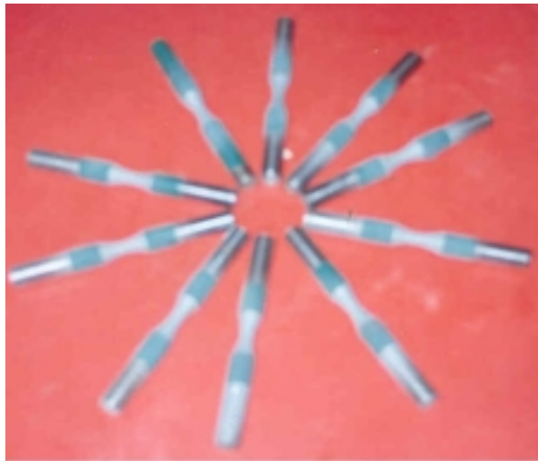
Fig.4 Sprayed samples for Fatigue test
