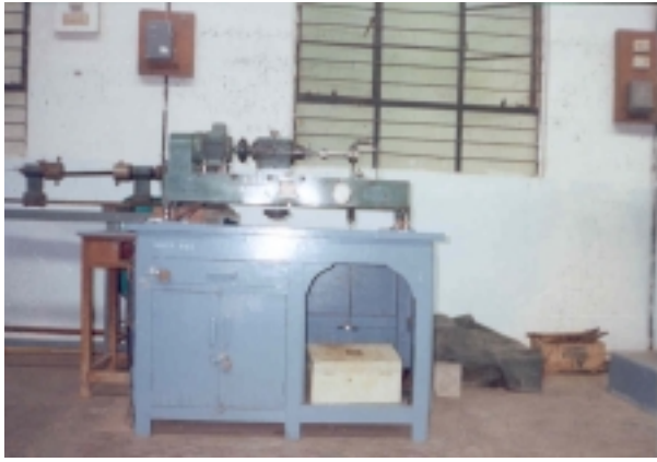
Fig.5 A typical rotating cantilever Fatigue Test Machine
