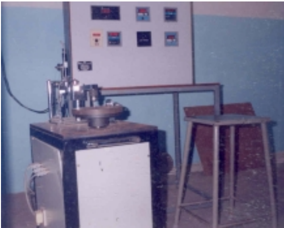
Fig.2 A typical pin-on-disc machine for wear testing
