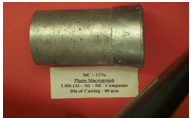
Fig. 6. Photo macrograph of Al-SiC Metal matrix Composite for macrostructure studies.
