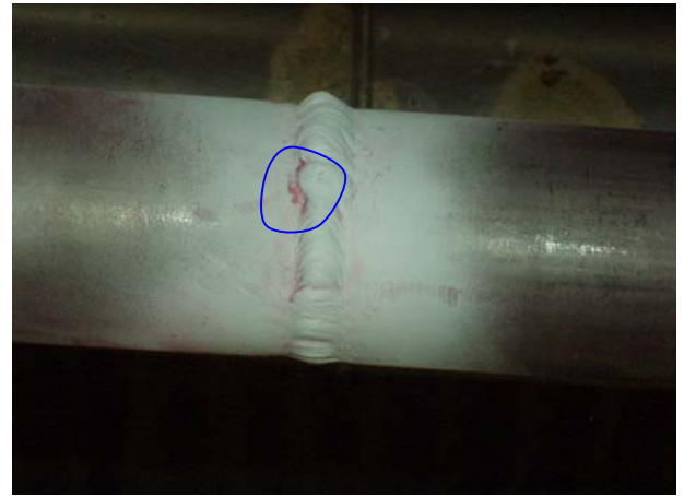
Figure 6- Photograph of Developer being applied on 2” stainless steel single butt weld
