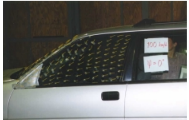
Fig 7. Side View of Flow Visualisation with Standard A-pillar, Yaw = 0°, Speed = 100 km/h
