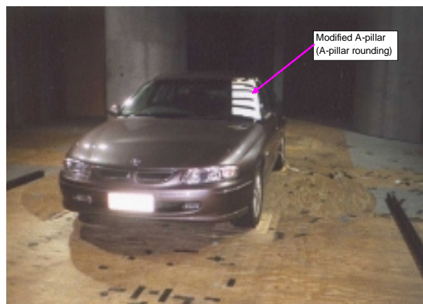
Fig 4. General Motors-Holden VT Calais with Modified A-pillar at Monash/RMIT Universities' Wind-Tunnel
