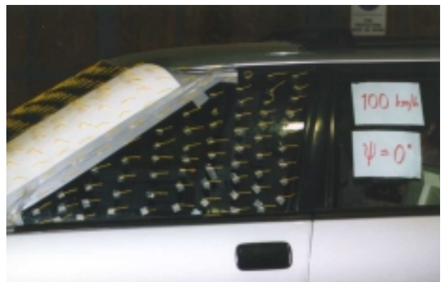
Fig 8. Side View of Flow Visualisation with Modified A-pillar, Yaw = 0°, Speed = 100 km/h
