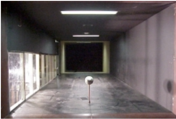
Fig 1. A Front View of Experimental Set Up with Rugby Ball in the Tunnel's Test Section
