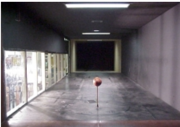
Fig 2. A Front View of Experimental Set Up with Australian Rules Football in the Tunnel's Test Section
