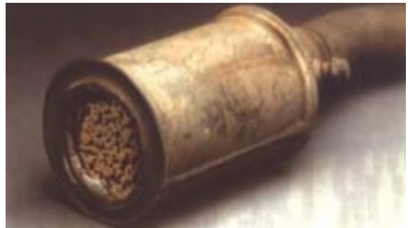
Fig-4c. Lubricating oil causing melting at the entrance
