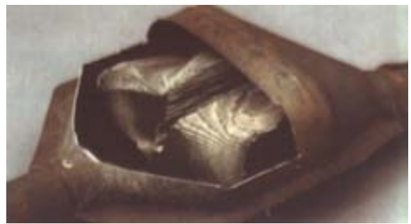
Fig-4d. CC damage due to mechanical breakage
