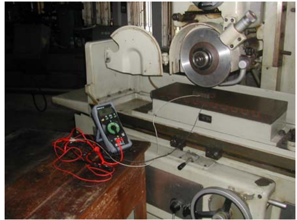
Fig 6. Methods of measuring the grinding temperature
