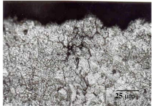
Fig 6. Optical microstructure showing intergranular cracks in failed forceps.
