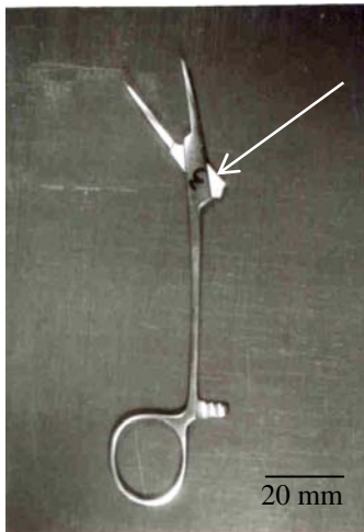
Fig 1(b). Fractured artery forceps (indicated by an arrow).
