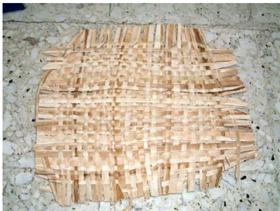
Fig 1. Pseudo-stem banana fibers in the woven fabric configuration
