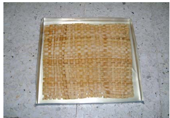
Fig 2. Pseudo-stem banana fibers reinforced epoxy composite during curing process
