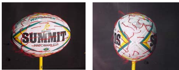
a) Flow Pattern at 0° Yaw b) Flow Pattern at 90° yaw
