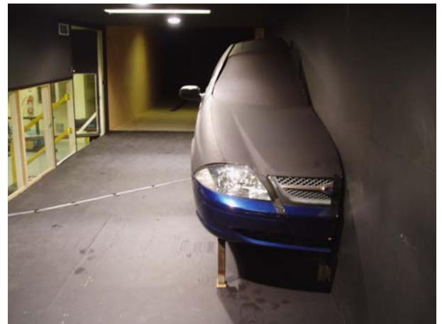
Fig 2. Experimental Set Up of the Quarter Model in Wind Tunnel
