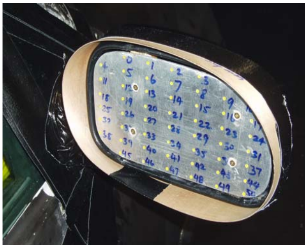
Fig 6. Modified Mirror with 44 mm Shrouding
