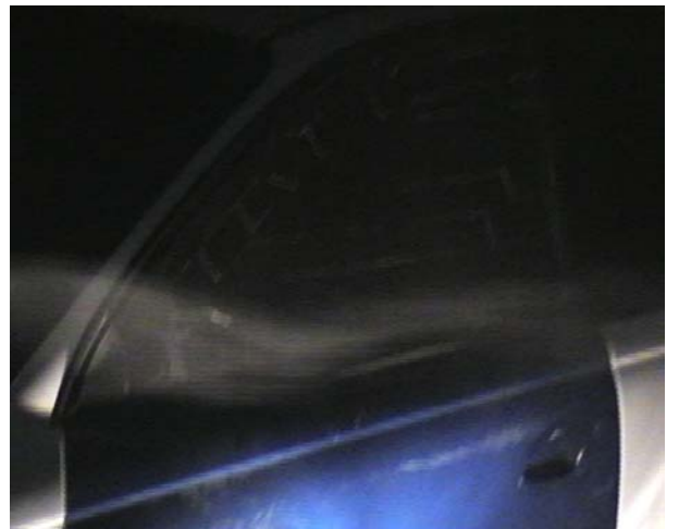
Fig 4. Flow visualization (smoke) 0^\circ yaw angle, No mirror, 1/4 pillar height
