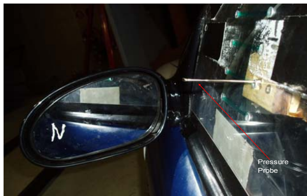
Fig 5. Mirror fitted, probe shown at position 3b, 50mm from window surface (Z=50 mm)
