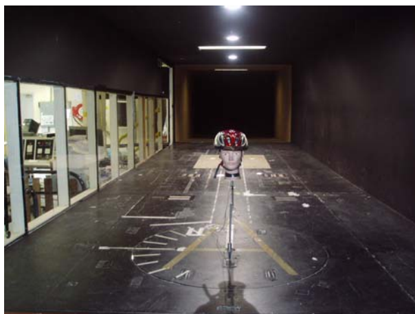
Fig 2. Experimental setup in the test section with a dummy head
