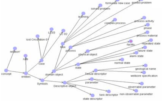
Fig 4: A part of the top-level ontology, showing concepts linked together with structural relations of type has subclass, each relation has its inverse ( here sub class of, not shown )
