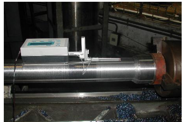
Fig 2: Photographic view of the surface roughness measuring technique
