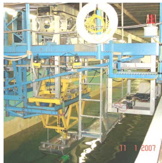
Fig 3: Pod dynamometer system installed on the OERC towing tank rails.
