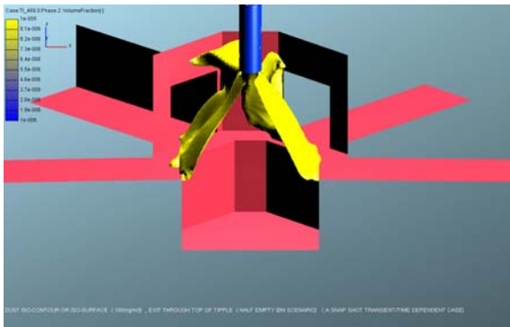
Fig 4(a): Dust iso-contours or iso-surface ( 100\text{mg}/\text{m}^3 ) (half-empty bin scenario) (A snap shot of transient/time dependent case)
