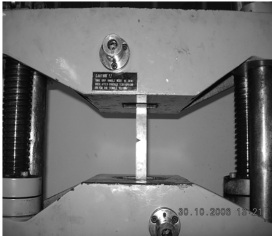
Fig 5: Specimen is loaded in Universal Testing Machine
