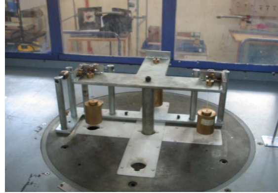
Fig 5: Calibration rig mounted the test section
