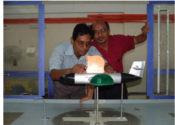
Fig 4: Aircraft model check for 0^\circ angle of attack.
