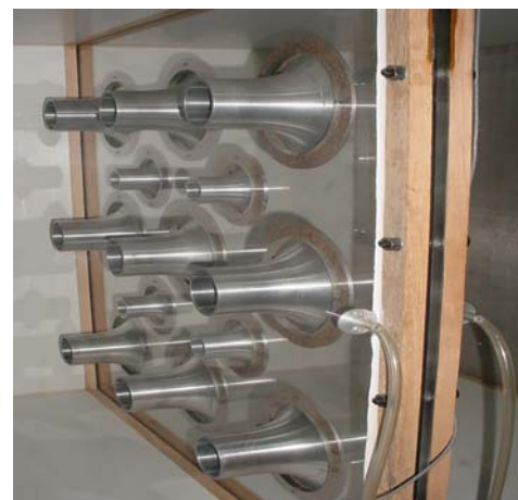
Fig 6: Photograph showing the back view of the set of nozzles in the test bed
