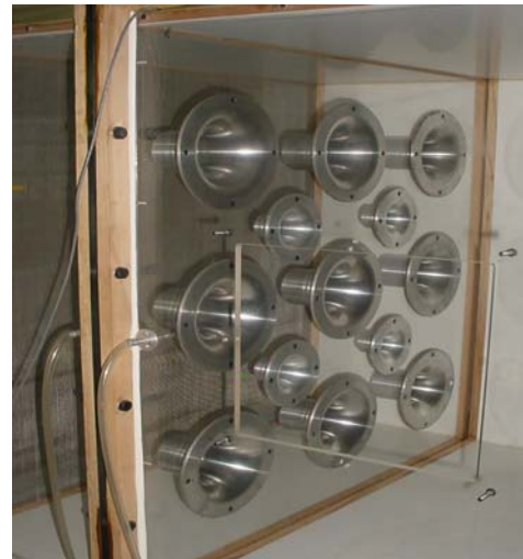
Fig 5: Photograph showing the front view of the set of nozzles in the test bed
