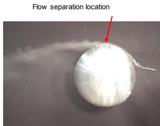
Fig 11: Seam orientation approximately 90 degrees with flow direction
