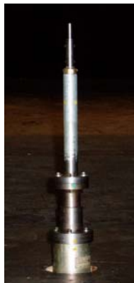
Fig 6: A Motorised Supporting Device for Cricket Ball mounted on a Six-Component Force Sensor
