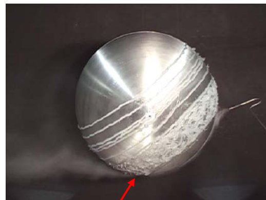
Fig 11: Seam orientation approximately 90 degrees with flow direction
