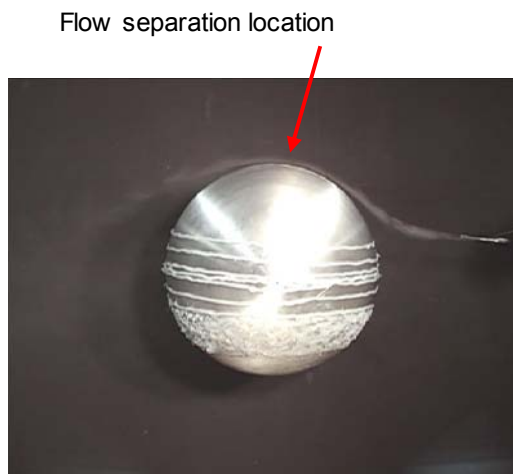
Fig 8: Seam orientation parallel to flow direction (0 degrees)
