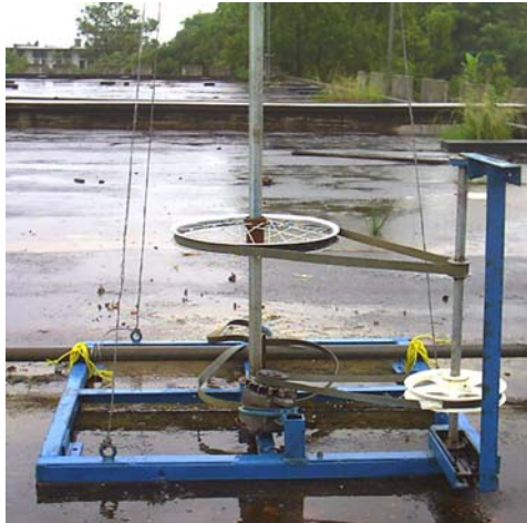
Fig 2: Photograph of the power transmission system
