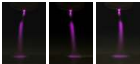
Figure 11. A sequence of images of the spinning discharge with deionized water as the anode at an electrode gap of 7.5 mm, each captured at an exposure time of 1/160 s.
