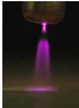
Figure 10. An image of the spinning discharge produced with deionized water as the anode at an electrode gap of 7.5 mm, captured with an exposure time of 1/60 s.
