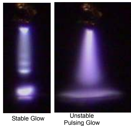
Figure 7. Image of stabilized and self pulsating glow discharges in hydrogen.
