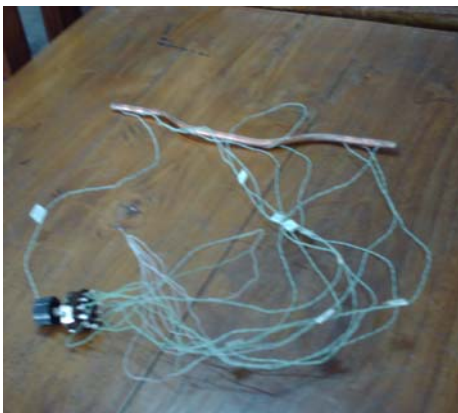
Fig 4: Arrangement of Thermocouple, Heat Pipe & Selector switch
