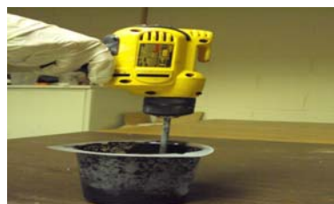
1c. Mechanical Mixing
