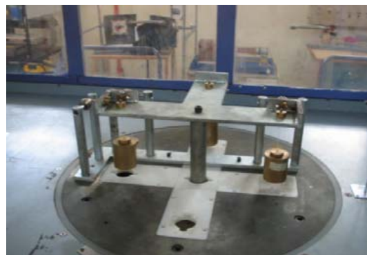
Fig. 2. Calibration rig mounted on the floor of the wind tunnel test section
