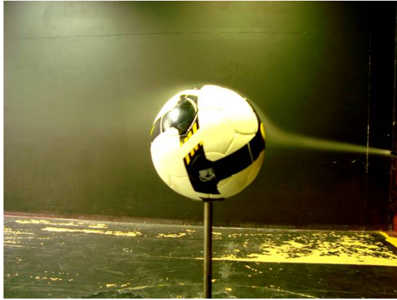
Fig 5. Airflow structure around a 32 panels football
