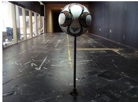
Fig 4. Experimental setup of a 14 panels football in the test section of RMIT Industrial Wind Tunnel
