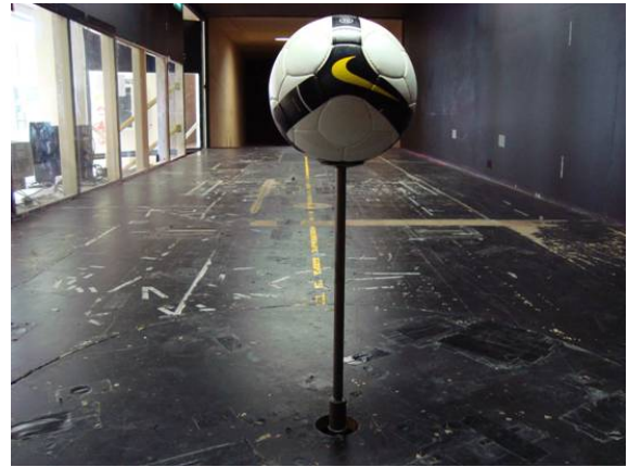
Fig 3. Experimental setup of a 32 panels football in the test section of RMIT Industrial Wind Tunnel
