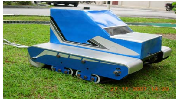
Fig 4. Developed prototype of hybrid electrical air-cushion track vehicle [8].
