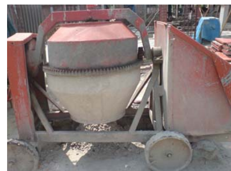
Fig 4b. Drive mechanism of a concrete mixer
