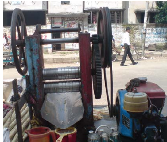
Fig 2a. Sugarcane Crushing Mechanism, Type-I
