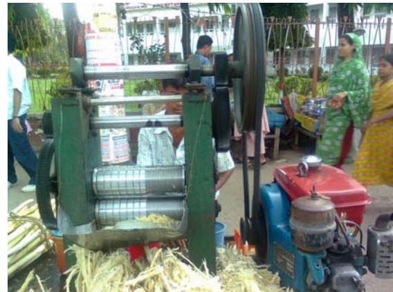
Fig 2b. Sugarcane crushing mechanism, Type-II
