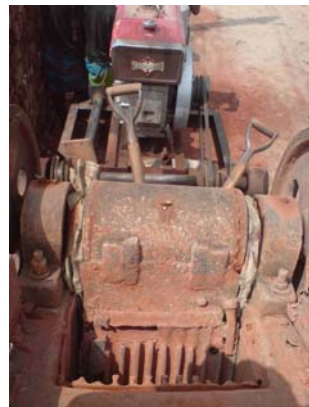
Fig 3b. Mechanism of a Brick Crusher
