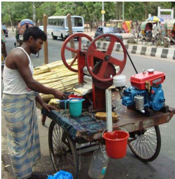
Fig 1. A 3-wheeler cycle-van mounted sugarcane crushing system used by roadside juice vendors
