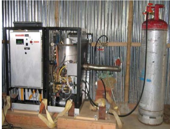
Fig 1. Experimental Set-up of DEKA Stirling Gen-set
