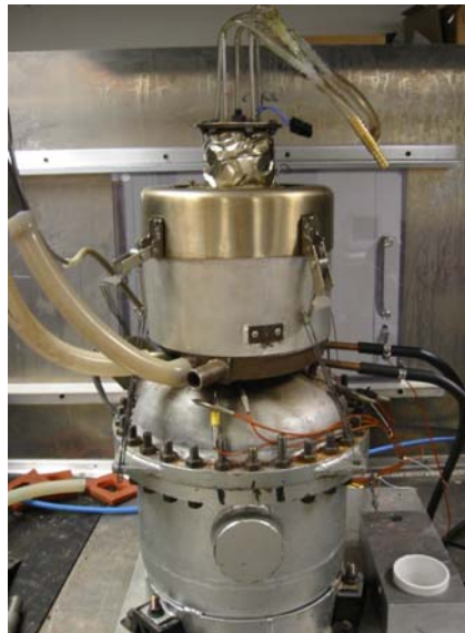
Fig 2. Components of the Stirling Engine
