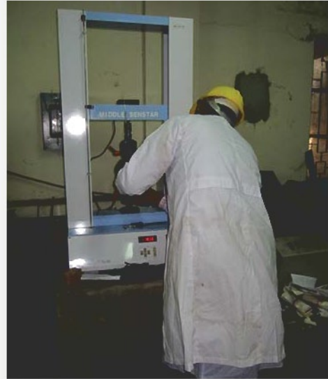
Desktop UTM (5 kN) for Rubber, Plastics and Soft Materials
