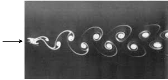
Fig. 3.1 von Karman vortex street behind a circular cylinder at Re = 300
