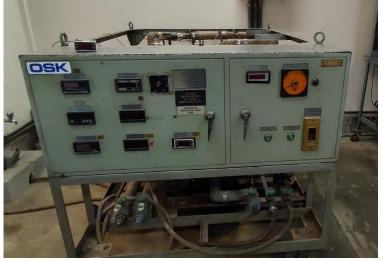
Front View of the Experimental Setup for Study and Performance Test of a Refrigeration Unit
