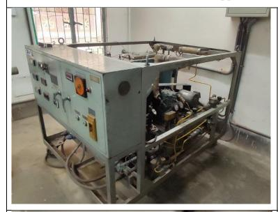
Experimental Setup for Study and Performance Test of a Refrigeration Unit
