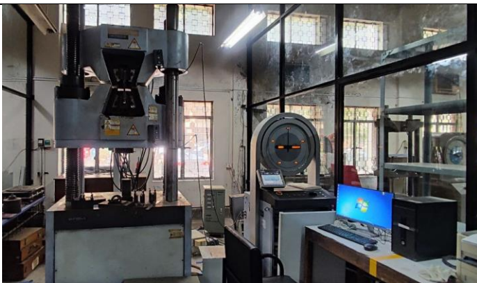
Experimental setup for Direct Shear Test of Metal
