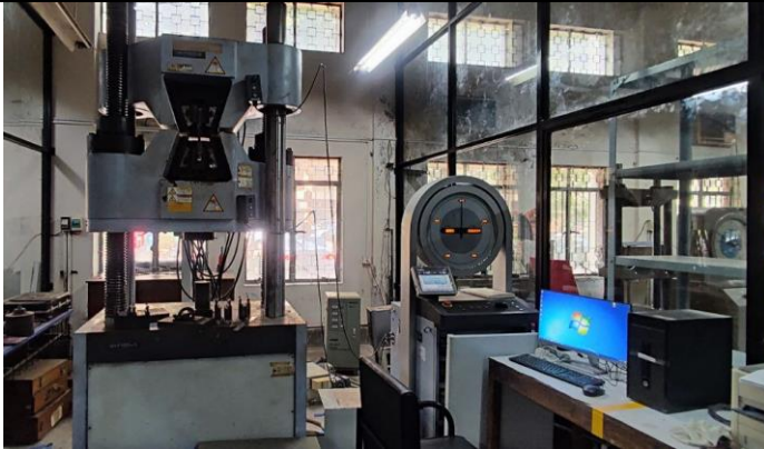
Experimental setup for Compression Test of Wooden Block
