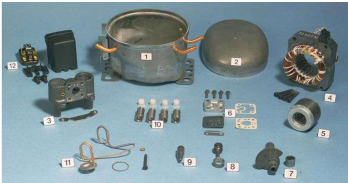
Figure 1(b): Various components of a Hermetically Sealed Compressor
